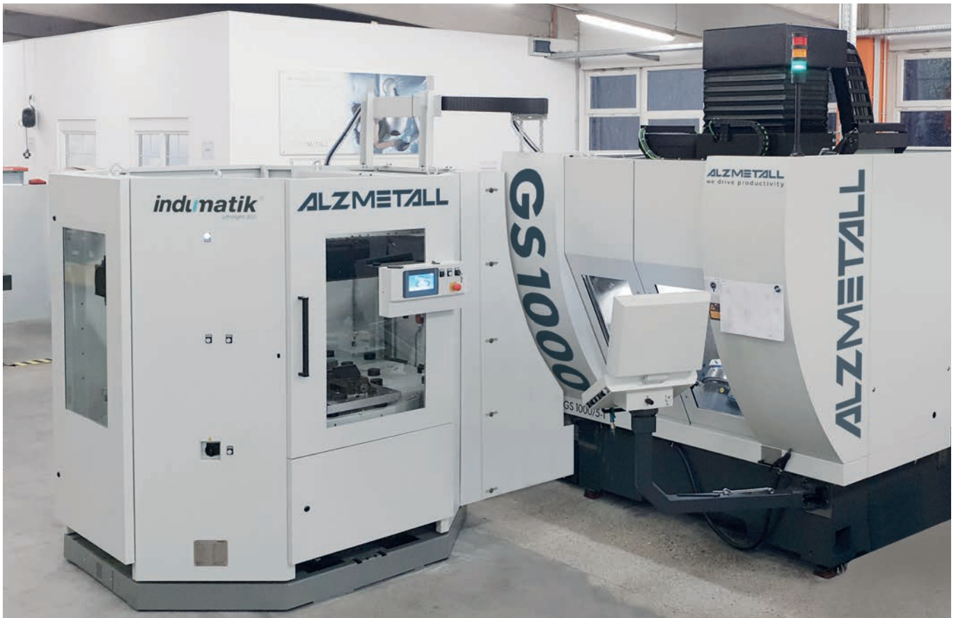
ALZMETALL GS 1000 and INDUMATIK Ultralight 300 implementation. Transfer weight of max. 300 kg, 3-12 pallet positions for pallets 320 x 320 mm up to 630 x 630 mm. Transfer carrier drive for operator access.
