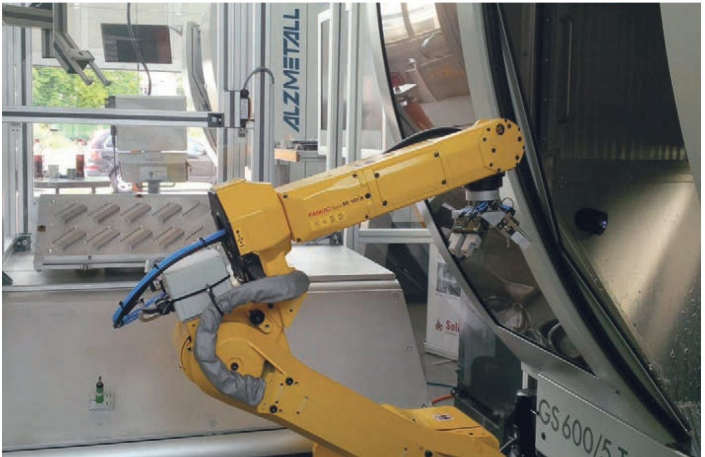
ALZMETALL GS 600/5-T and WU-robot cell RZ-3/20 implementation for specific part handling. Transfer weight of 20 kg dependent on inserted gripper.
